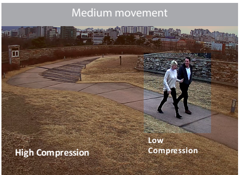
WiseStream II OFF : 7260kbps WiseStream II ON : 2901kbps
